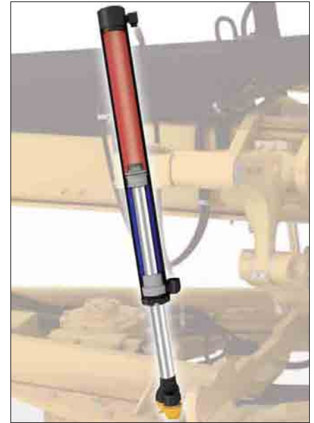
Blade lift cylinder: red = 40 liter/min, blue = 24 liter/min
